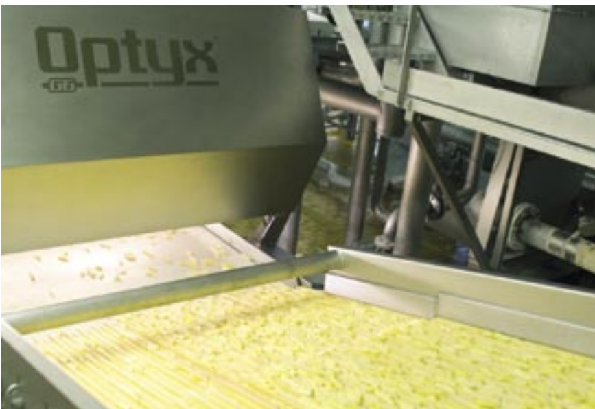
Infeed to Optyx of potato strips
