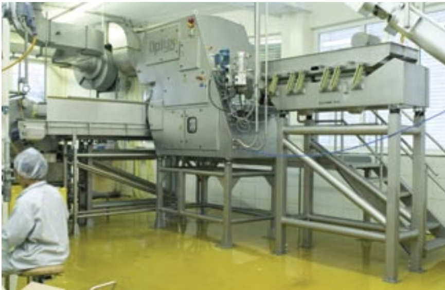
Optyx in use on shredded potato line
