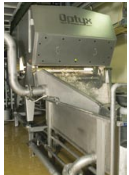
Discharge from Optyx on potato strip line
