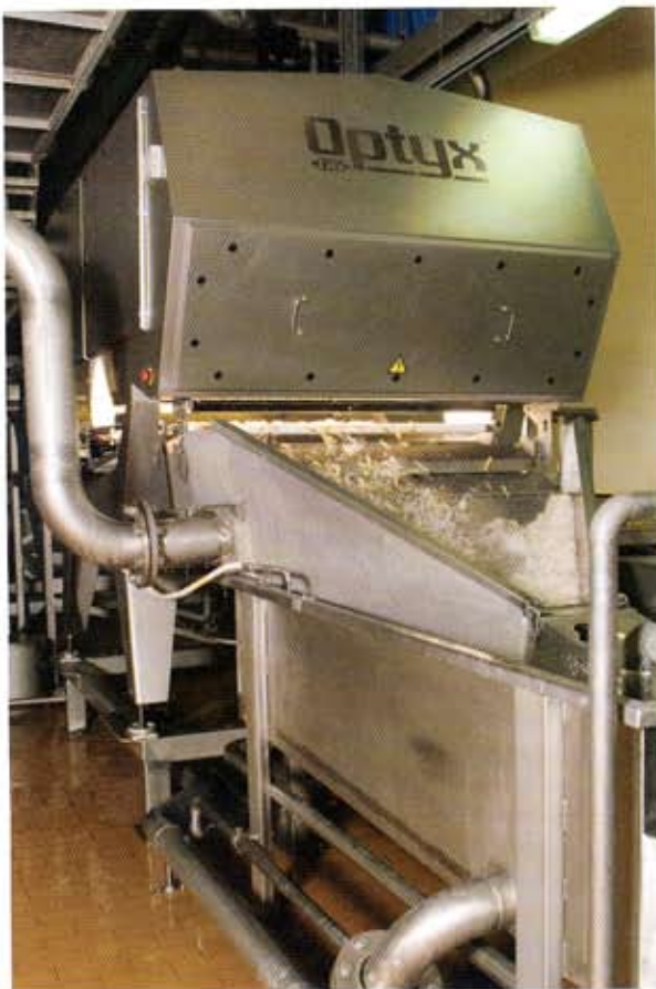
The discharge end of the Optyx sorting system.
