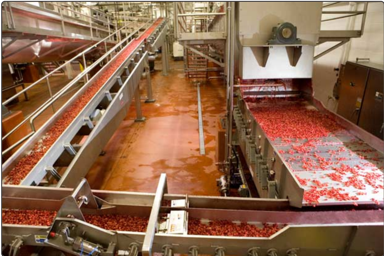
Iso-Flo vibratory shakers form an integral part of the sanitary Ocean Spray processing line.
